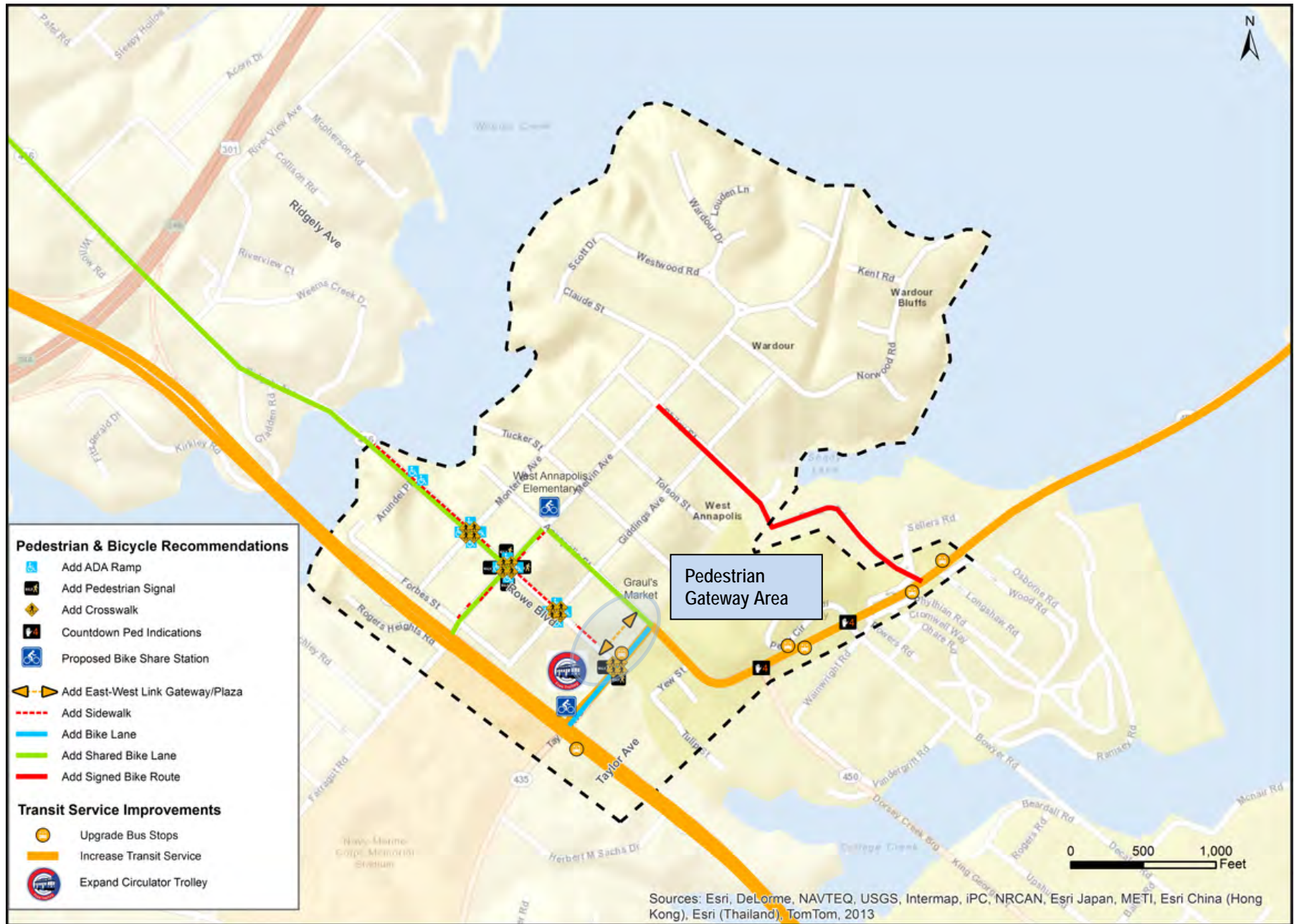
Figure 2.24: Recommended Pedestrian, Bicycle and Transit Improvements
