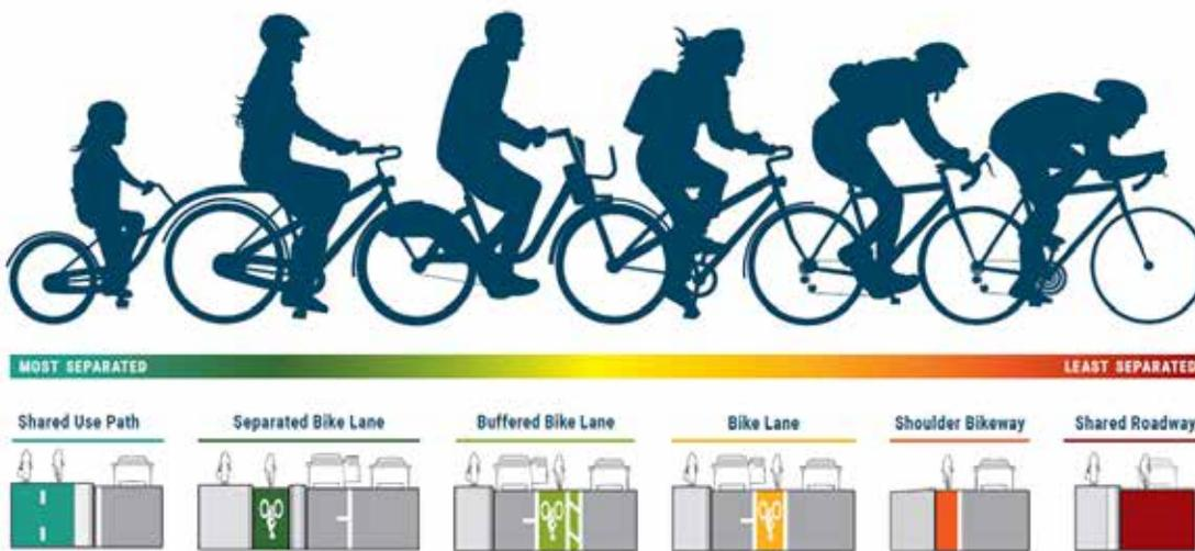
**FIGURE 11-16: BIKE FACILITIES RANGE DRAMATICALLY IN REGARD TO HOW SEPERATED THEY ARE FROM VEHICULAR TRAFFIC AND REFLECT THE TYPES OF CYCLISTS WHO WILL FEEL SAFE ON THE FACILITY.**
