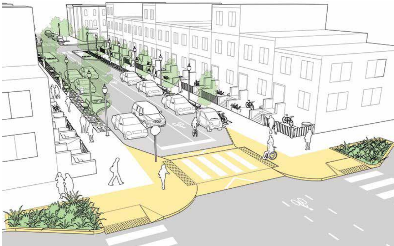
FIGURE 6-15: RENDERING OF A PROTOTYPICAL NEIGHBORHOOD COMPLETE STREET FROM THE 'URBAN STREET DESIGN GUIDE' BY THE NATIONAL ASSOCIATION OF CITY TRANSPORTATION OFFICIALS (NACTO)
