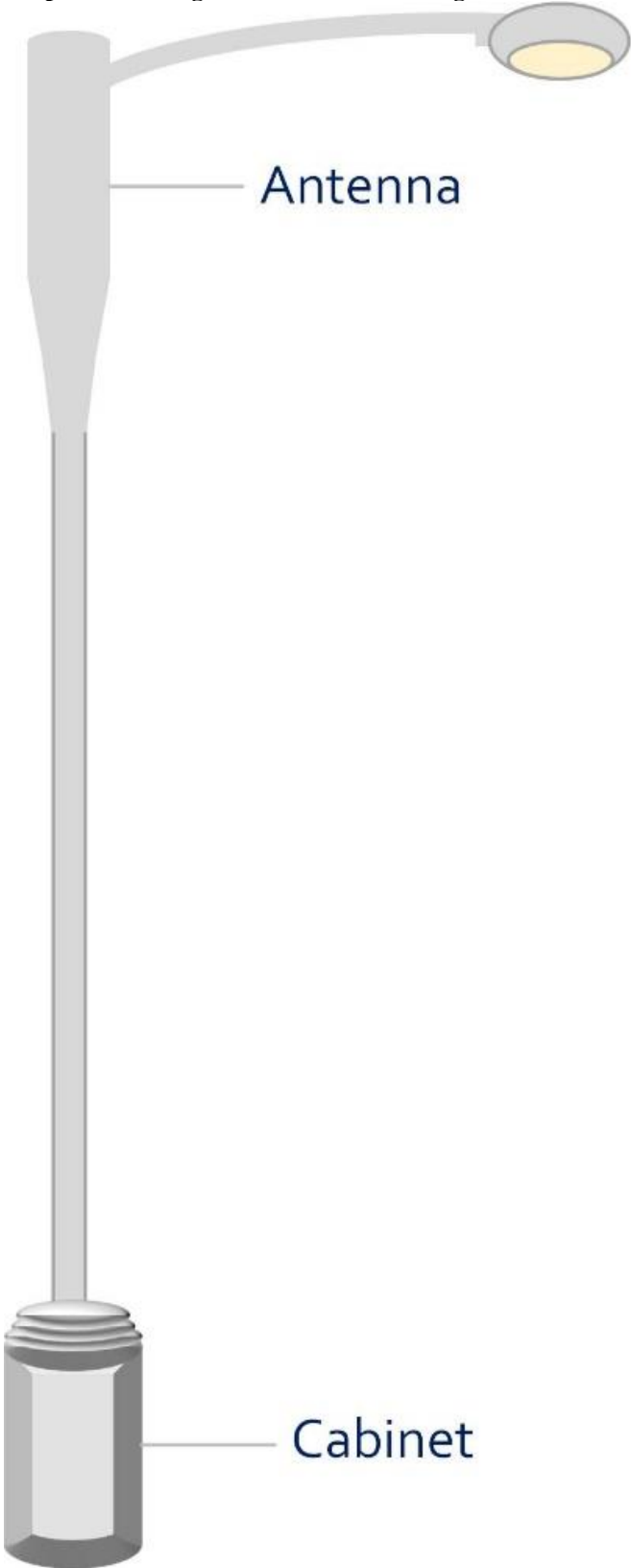
Figure 3: Conceptual Drawing of a Small Cell on a Light Pole with Concealed Cabinet
