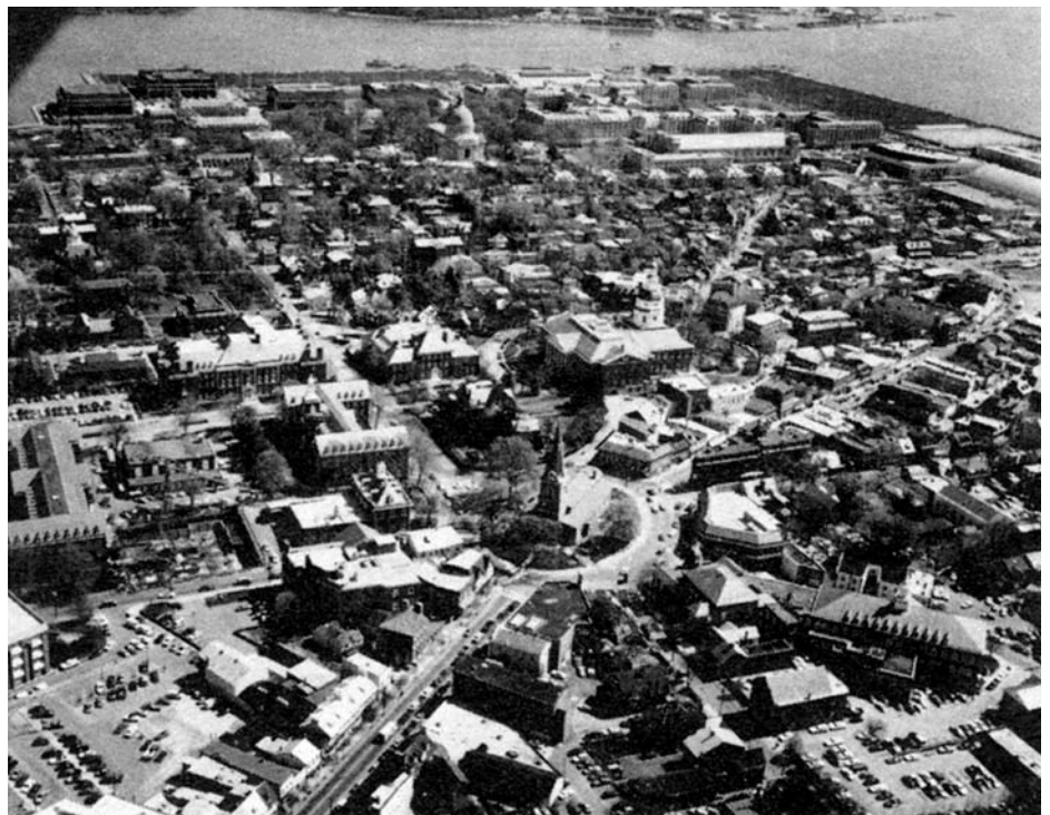
Figure 56. Aerial view of Annapolis. The radiating streets of the original town plan opened on to the water or an orthogonal street at one end, and were closed by State Circle or Church Circle at the other. (Photograph courtesy of Kevin Fleming)
