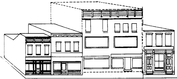
NO The large mass and size of this new building are not compatible with its immediate neighborhood.
