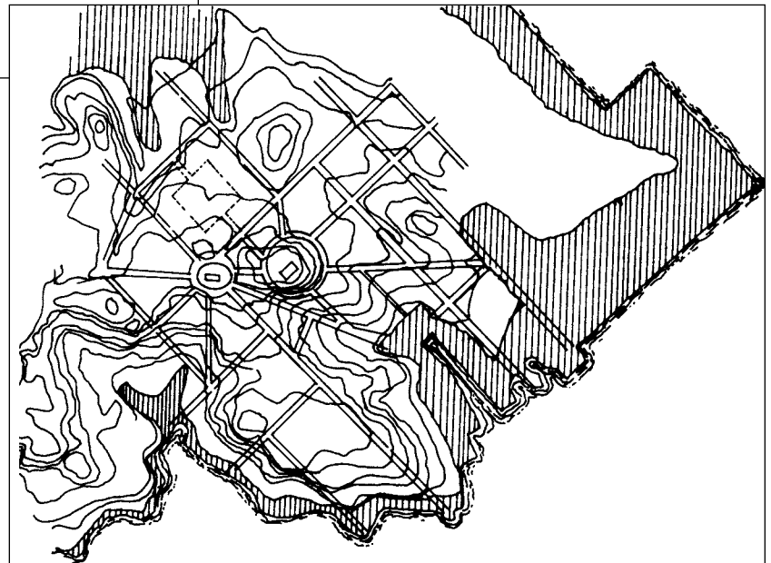
Figure 10 (below). Map of the original water's edge outline. This generalized topographic map reveals how the urban form was made to fit the natural land form, with the two circles placed on the highest points. The water's edge has been altered by land infill. Note how Main Street follows a valley from Church Circle, and East Street follows a ridge from State Circle.
