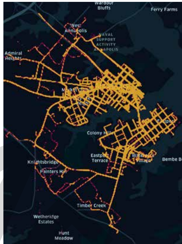
FIGURE 6-22: USING RIDER DATA PROVIDED BY BIRD, THE MAP ABOVE SHOWS THE ROADWAYS MOST USED BY E-BIKES AND E-SCOOTERS IN A TYPICAL WEEK AND CAN HELP TO PRIORITIZE ROADWAY IMPROVEMENTS FOR ACTIVE TRANSPORTATION
