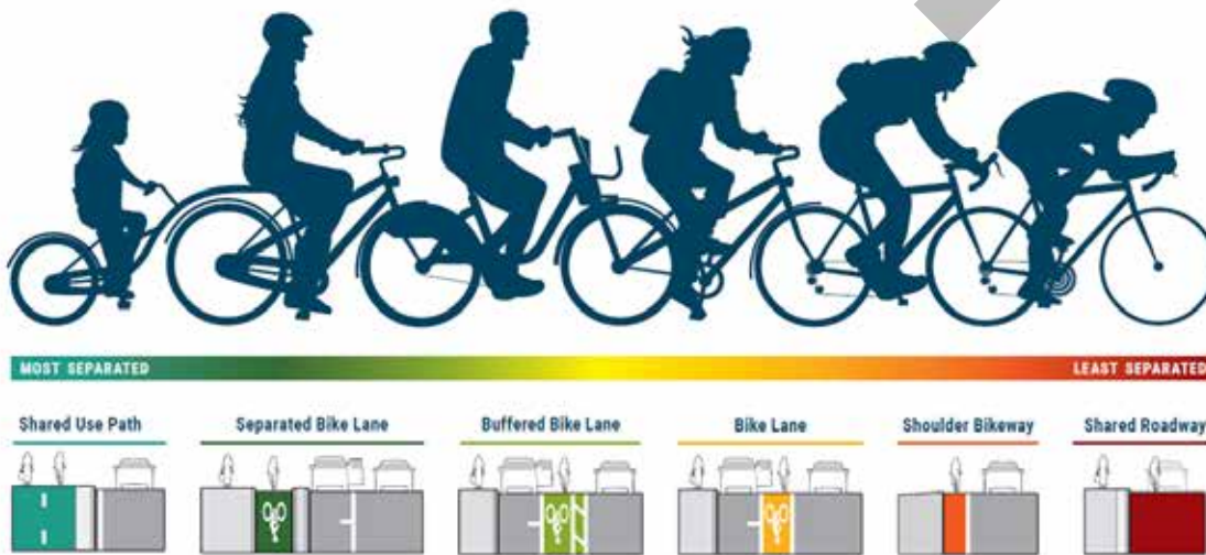
FIGURE EX-42: BIKE FACILITIES RANGE DRAMATICALLY IN REGARD TO HOW SEPERATED THEY ARE FROM VEHICULAR TRAFFIC AND REFLECT THE TYPES OF CYCLISTS WHO WILL FEEL SAFE ON THE FACILITY.
