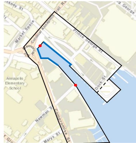
Fig 1. Black lines represent the delimited scoped area. Red dots represent lowest elevation areas at the dock, with the left upper red marker being at a 1.5 ft NAVD88 elevation and the right most point at a 1.80 ft NAVD88 elevation. Blue solid lines represent the current concrete bulkheads (sea wall) at about 4.65 ft NAVD88. Dashed black line delimited the end of dock street. (Source image from Google maps).
